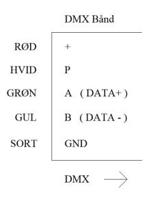
Connect as shown on picture. Feed +24V direct to tape and GND to both controller and tape. (colors for wires can be different for your tape-type.
