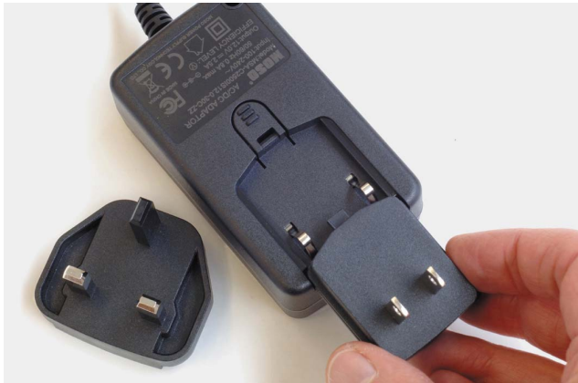
Fig. 1. Fit the appropriate plug to the Power Supply Unit and connect the PSU to a suitable AC supply (100-240V See Specification 2.7).
