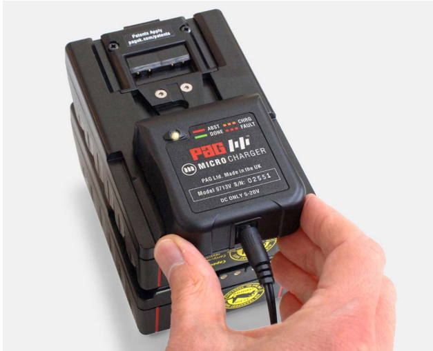
Fig. 3A. Slide the V-Mount Micro Charger over the contacts on the rear of the V-Mount battery.
