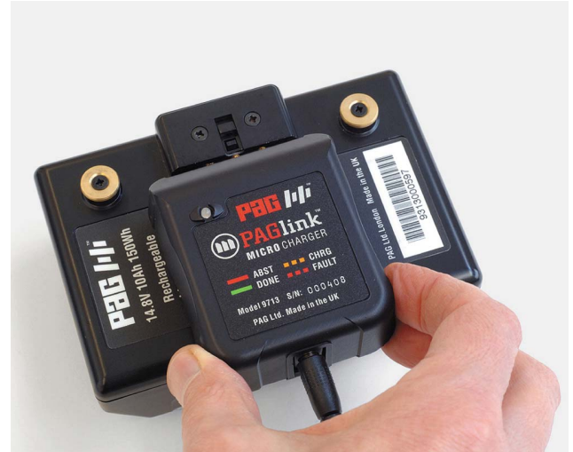
Fig. 3B. Slide the Gold Mount Micro Charger over the contacts on the rear of the Gold Mount battery.
