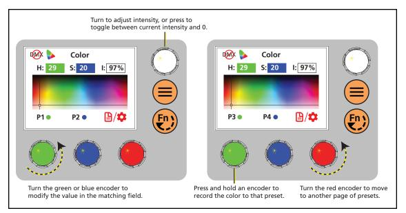
2. Turn the encoders to change the corresponding values. For example, turn the Intensity encoder to change the intensity value, or turn the green encoder to change the hue value. The crosshairs on the display indicate the approximate color.
