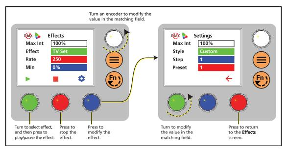
2. Turn the green encoder to select an effect, and then press the encoder to play the effect.
