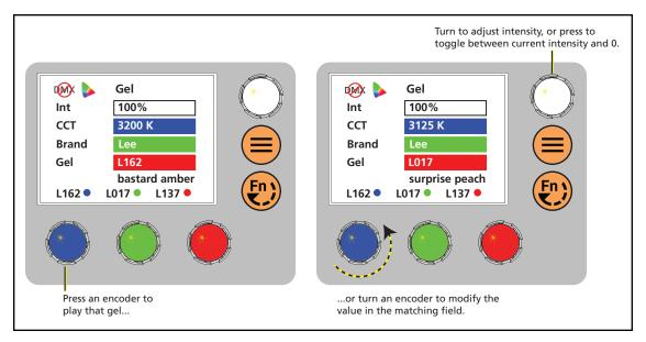
2. Turn the encoders to change the corresponding values. For example, turn the red encoder to change the **Gel** value, or turn the blue encoder to change the **CCT** value.
