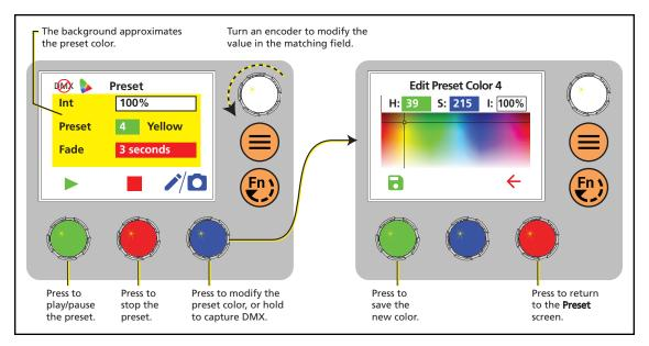
2. Turn the green encoder to select a preset, and then press the encoder to play the preset.
