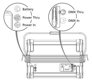
Power Thru: Link a small (PL8 or PD8) fixture to up to three other small fixtures, or link a medium (PL16 or PD16) fixture to another medium fixture via Power Thru connector when using an R20 Relay Module, ER15 Relay Module, or Unison Echo Relay Panel (consult breaker-trip curves when using other equipment). When linking other combinations of fixtures, do not exceed the rating of the power connectors (20 A in 120 V/60 Hz regions and 16 A in 240 V/50 Hz regions).
