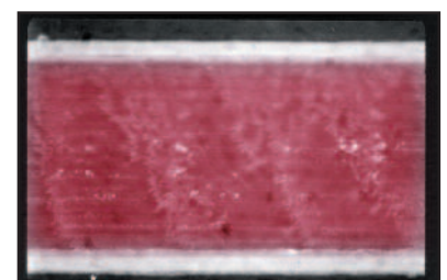
Shown here is a cross section of co-extruded Rosco Supergel filter photographed through an electron microscope. Note the discrete clear layers on the top and bottom sealing in the colour core.
